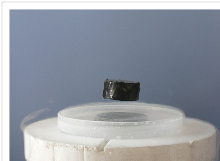
The Meissner effect causes a magnet to levitate above a superconductor
